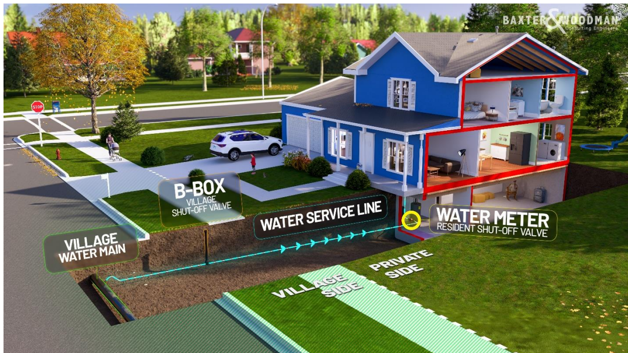
Figure 3 - Water Service Line Ownership
